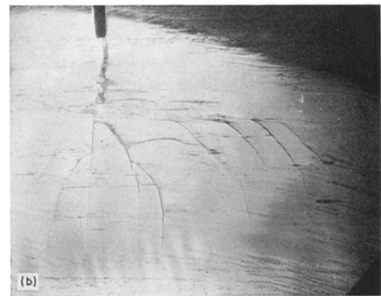
Figure 6 A section through a notched tensile specimen—(a) viewed under oblique illumination and (b) viewed under normal illumination.
